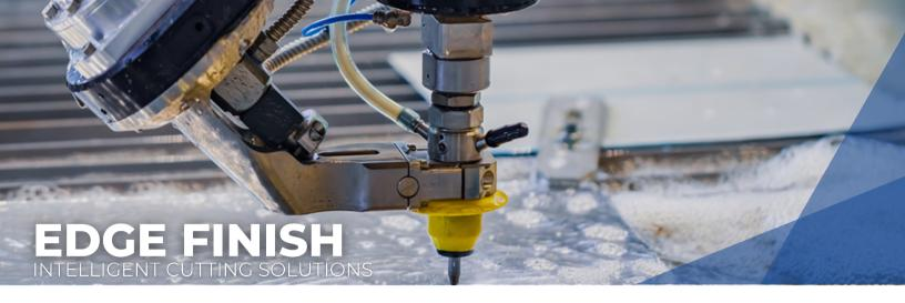
Intelligent Cutting Solutions (ICS) offers four levels of surface finish so you can get exactly what you need. Each finish is associated with a specific cutting speed, the smoother the surface finish the longer the cutting time.
